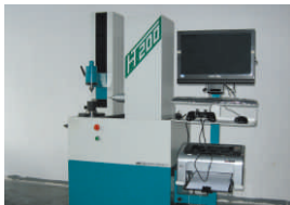
Full-automatic Gear Testing Apparatus 全自动齿轮检测仪
