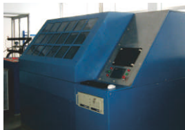
Testing Platform of Pressure Impulse 压力脉冲测试台
