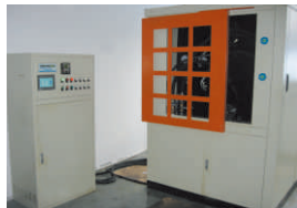
Testing Platform of Gear Pump 齿轮泵测试台
