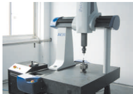
Full-automatic Three-dimensional Measuring Apparatus 全自动三坐标测量仪
