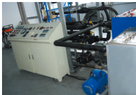
Capability Testing Platform of radiators 散热器性能测试台
